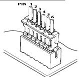
Compatible speed control must use the six position JST header part number X-6B-ZR-SMX-TK (where the X denotes the style of the header), or equivalent.
