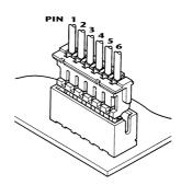
Sensored type compatible speed controls must use the six position JST header part number X-6B-ZRSMX-TK (where X denotes the style of the header) or equivalent. The power motor wire connections must be clearly marked A, B, C on both speed control and motor.
