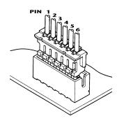
Sensored type compatible speed controls must use the six position JST header part number X-6B-ZRSMX-TK (where X denotes the style of the header) or equivalent. The power motor wire connections must be clearly marked A, B, C on both speed control and motor.
