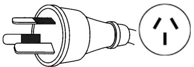
The diagram above indicates the shape of an Australian domestic power plug, this type of plug is unique to Australia. Ensure that your equipment is also able to handle the lower cyclic rate of 50 Hz, most 240v countries are at 60Hz. Generally this is only a problem with electric clocks and things of this nature.
